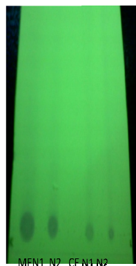
Fig.2: Observation of TLC in UV before vanillin spray
